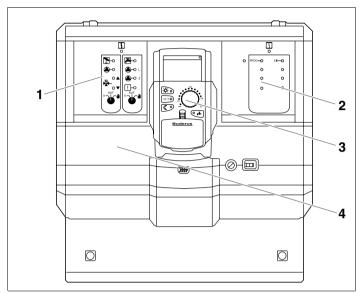
Fig. 3 Function module FM 446 inside the Logamatic 4112 control device
